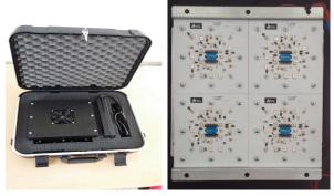
The Hyperion Solar Simulator is a unique piece of equipment in the solar light emulation environment. It is the perfect joint between the best qualities of a standard high performing solar simulator and a long life light soaker with the addition of peculiar characteristics that only LED technology can give.
